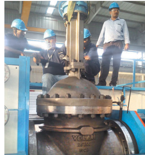
Performance testing of a 24" (600 mm) cast steel gate valve manufactured in India.
