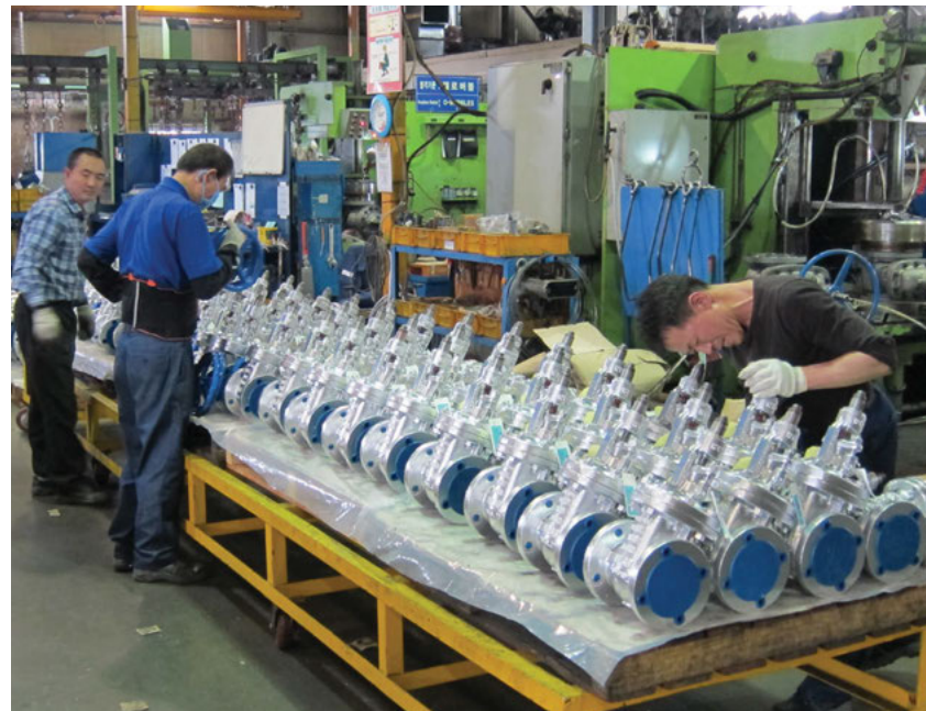
Inspection and assembly of gate valves
